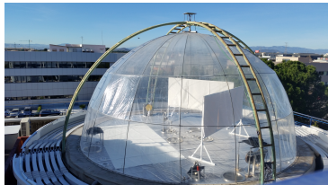
Atmospheric simulation chamber. Illustration Eurochamp website, EUPHORE (Spain)
